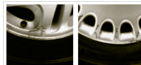
EXCESSIVE: wheel-cover damage
