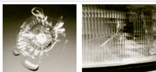
EXCESSIVE: cracked windshield
