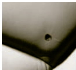
EXCESSIVE: upholstery burn
