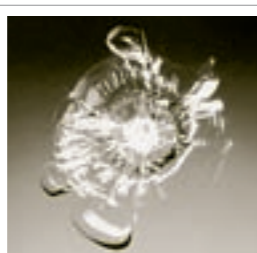
EXCESSIVE: cracked windshield
