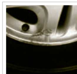
EXCESSIVE: wheel-cover damage
