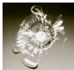
EXCESSIVE : pare-brise fissuré
